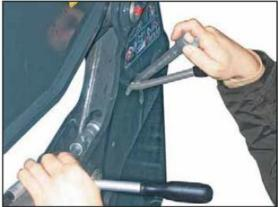
To set the lock, you will need an open-ended spanner (WAF 24), a  $\frac{1}{2}$ " ratchet with the corresponding extension, joint and 24 mm socket spanner.
