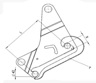
On the drive-in hook, check the front carriage of the 40 mm shaft and the hook (dimension of X max 63.2 mm). The hook is supplied as a weld-on part as a spare part.
